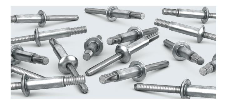
HUCKLOK™ blind rivets are especially high-strength blind rivets with a very wide gripping range that remain snug even under dynamic load. The mandrel always breaks flush, even when materials of varying strengths and thicknesses are present within the grip range. The blind-side footprint is minimal.
