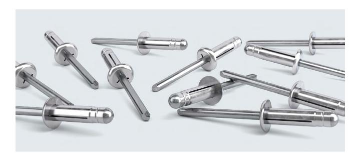
POP® LSR folding leg blind rivets with load-distributing properties are especially suited for use on soft, fragile or brittle materials. They fit very snugly and securely in metal/plastic fastenings and have a very large grip range. The folding sleeve expands into three legs on the blind side. This claw technique creates a large contact surface on the blind side. The contact load distributes across the rear material and provides high pull-out resistance.
