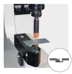
Clinching / Metal joining: This method replaces the conventional spot welding of thin sheeting.
