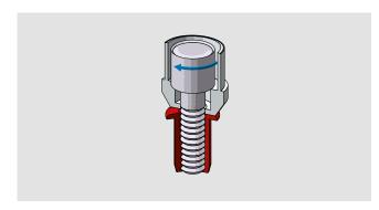
Insert the RIV-TI\* blind rivet nut into the pre-drilled hole.
