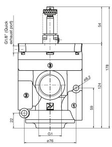
For vacuum - N.O. Exhaust port 3 Outlet port 2 Pump 1
