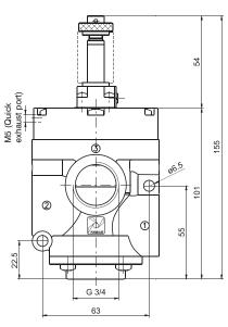
For compressed air - N.C. Inlet port 1 Outlet port 2 Exhaust port 3
