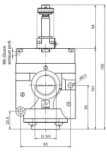
For vacuum - N.O. Outlet port 1 Outlet port 2 Pump 3
