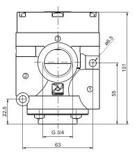
For vacuum - N.C. Exhaust port 3 Outlet port 2 Pump 1
