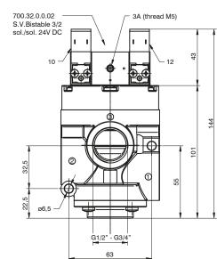
For compressed air - N.C. Inlet port 1 Outlet port 2 Exhaust port 3
