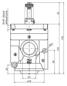
For compressed air - N.C. Inlet port 1 Outlet port 2 Exhaust port 3
