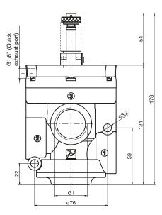
For compressed air - N.C. Inlet port 1 Outlet port 2
