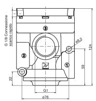
For vacuum - N.C. Exhaust port 3 Outlet port 2 Pump 1
