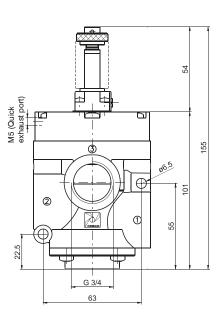
For vacuum - N.O. Exhaust port 3 Outlet port 2 Pump 1
