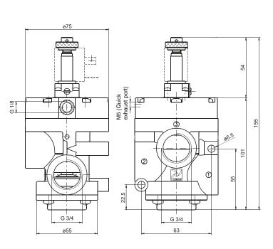
For vacuum - N.O. Outlet port 1 Outlet port 2 Pump 3
