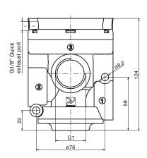
For compressed air - N.C. Inlet port 1 Outlet port 2 Exhaust port 3
