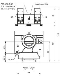
For vacuum - N.C. Pump 1 Outlet port 2 Exhaust port 3
