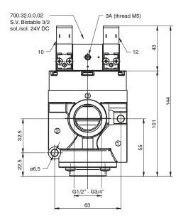
For vacuum - N.C. Pump 1 Outlet port 2 Exhaust port 3
