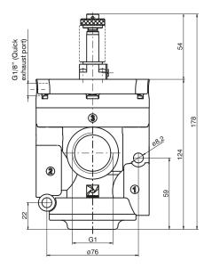
For vacuum - N.O. Pump 3 Outlet port 2 Outlet port 1
