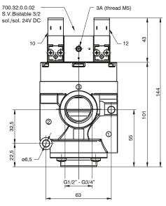
For compressed air - N.C. Inlet port 1 Outlet port 2
