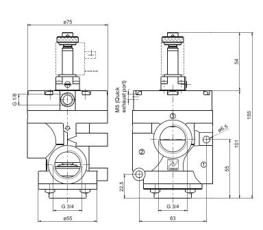
For compressed air - N.C. Inlet port 1 Outlet port 2 Exhaust port 3
