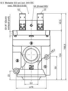
Minimum piloting pressure 2.5 bar
